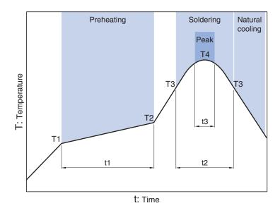
Preheating Soldering Peak Temp. Time Temp. Time Temp. Time T2 T4 t3 150°C 180°C 90 to 120s 40s 230°C 255°C 10s max.
